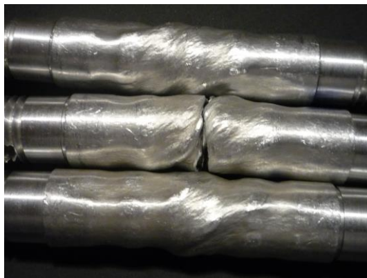
Fig. 3 Joints deformed and fractured by torque
